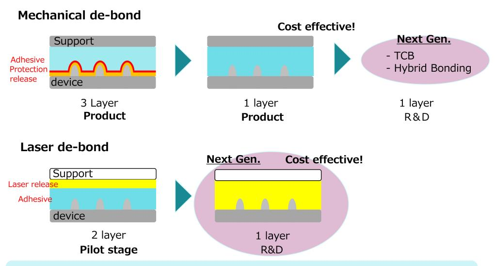
NCC have Supported HVM in customer for ~HBM2 and developing next Gen. mechanical and laser de-bonding materials.
