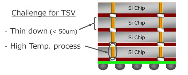
Special handling process and materials are necessary for wafer thin down process.
